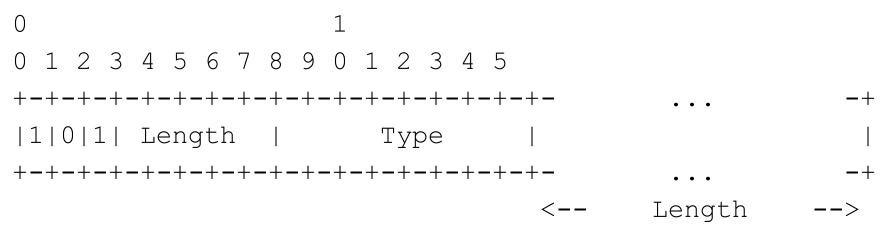
Elective format (above) is skippable thanks to standard length field whereas Critical format is not. Length is derived from Type/ Type Specific Extension
