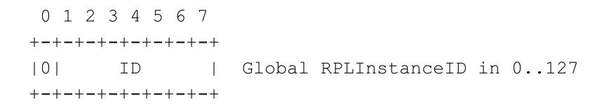
For the global Instance 0, the RPLInstanceID field is all zeroes Define 'I' flag that, when set, signals a global Instance 0, elided.
